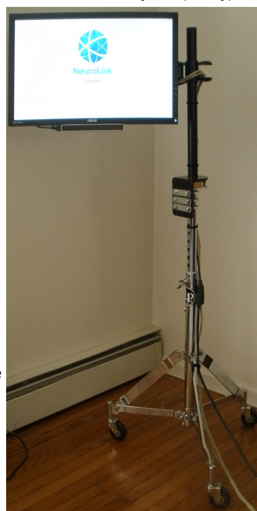
The EyeTribe eye-tracker is attached to the bottom of the monitor in the photo of the prototype shown above.
